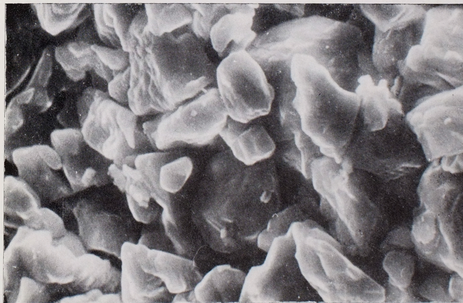
Phot. 6. Aggregates of tabular gorceixite crystals. SEM, 1400\times . Phot. E. Klichowicz
