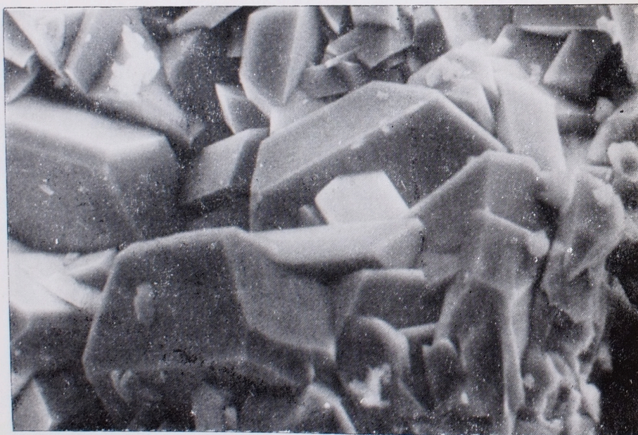
Phot. 8. Gorceixite aggregate. Crystals exhibit a prismatic-rhombohedral habit. Largest grains are 0.05—0.06 mm in diameter. SEM, 800 \times . Phot. E. Klichowicz
