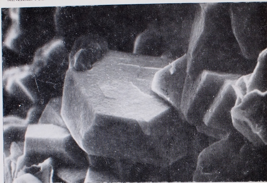
Phot. 7. Gorceixite aggregate. A crystal in the centre of aggregate, about 0.03 mm in size, shows distinct trigonal symmetry. SEM, 2000 \times . Phot. E. Klichowicz
